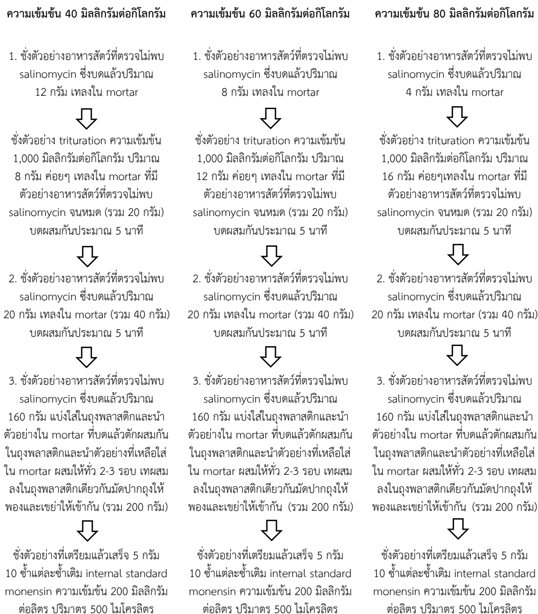
Fig. 3. The preparation of matrix-fortified sample for testing of homogeneity.
