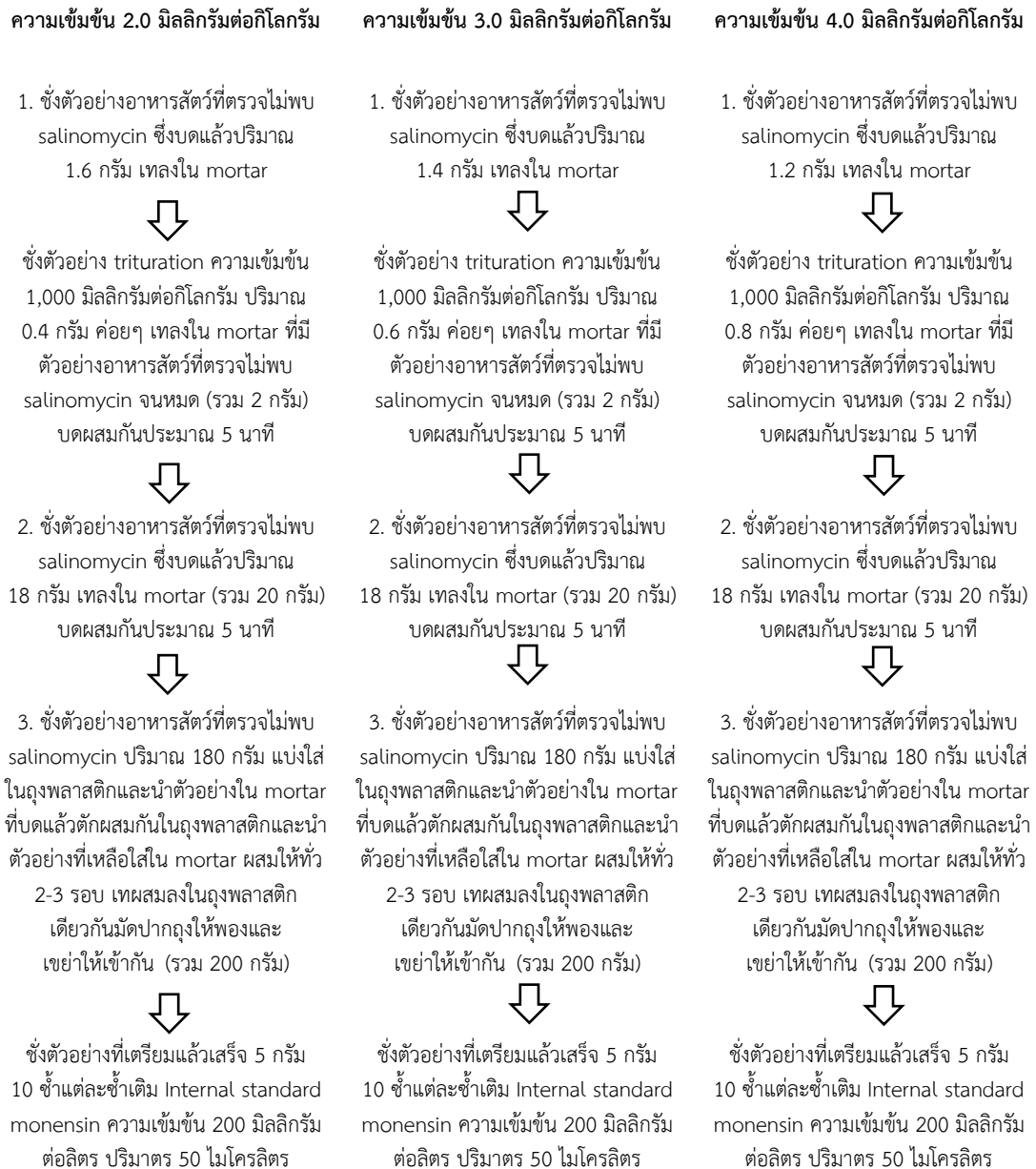
Fig. 4. The preparation of matrix-fortified sample for testing of drug carryover.
